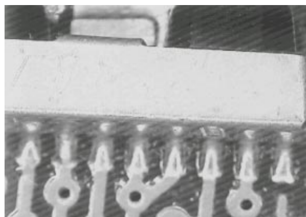
Photo 4.0. Unit self-aligns after reflow.
