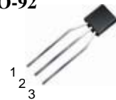
1.Gate 2. Drain 3. Source
