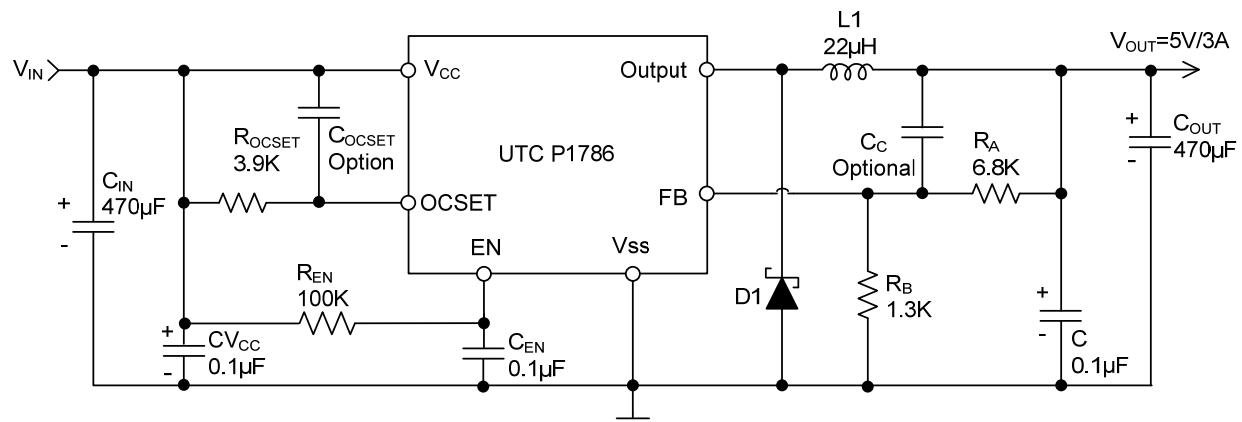
Note:  $V_{OUT} = V_{FB} \times (1 + R_A/R_B)$ ,  $R_B = 0.7K \sim 5K$  ohm
