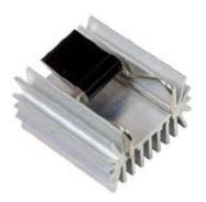
Ohmite's R2 Series (patent pending) heatsink provides a large surface area along with our C Series clipping mechanism to attach either a T0-220 or T0-247 package. The self-aligning features of the clip assure secure attachment and enhanced thermal performance. Because no screws are required for device mounting, additional fins can be added to the rear side of the heatsink for increased total surface area in a more compact space.
