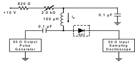
Notes: 1. A 2.0k $\Omega$  variable resistor adjusted for a forward current (I<sub>F</sub>) to 10mA 2. Input pulse is adjusted to I<sub>R(peak)</sub> is equal to 10mA
