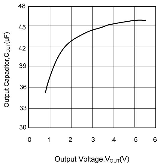
Maximum Output Capacitor's Changing Over  $V_{OUT}$ .
