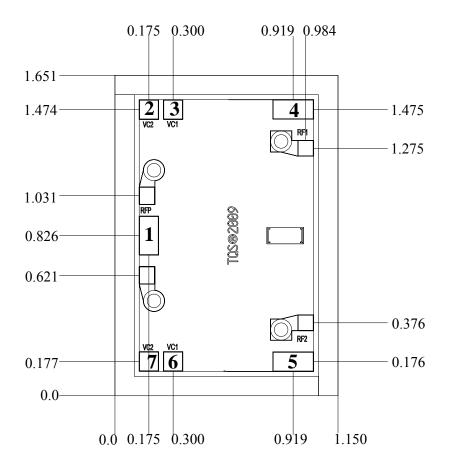
Unit: millimeters Thickness: 0.10
