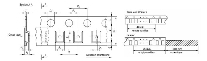
Dimensions and tolerances in mm:
