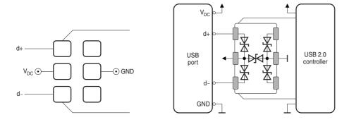
Note: USB 2.0 single port line protection with high-speed array CDA6C05GTA.
