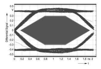
Note: USB 2.0 compliance test result of high-speed array CDA6C05GTA.
