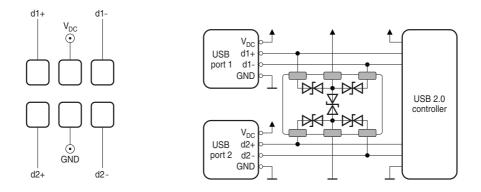
Note: USB 2.0 dual port line protection with high-speed array CDA6C05GTA.
