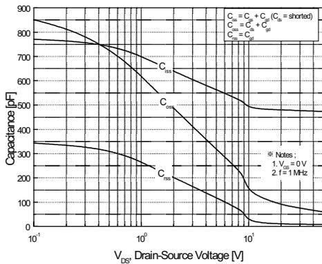
Figure 5. Capacitance Characteristics
