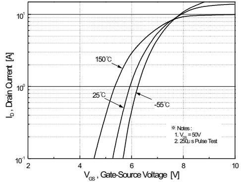
Figure 2. Transfer Characteristics
