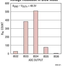
ADC Integral Nonlinearity Voltage Readback in Slow Mode
