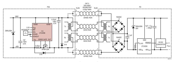
Figure 10. Power Over Ethernet System Diagram
