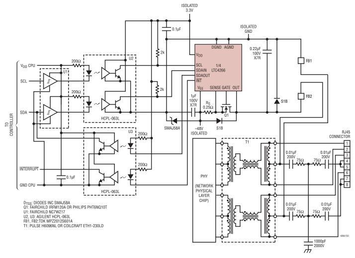
Figure 22. One Complete Isolated Powered Etherent Port
