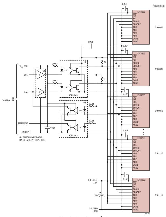
Figure 18. Opto-Isolating the I<sup>2</sup>C Bus
