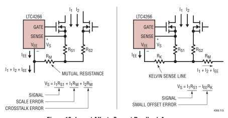
Figure 19. Layout Affects Current Readback Accuracy
