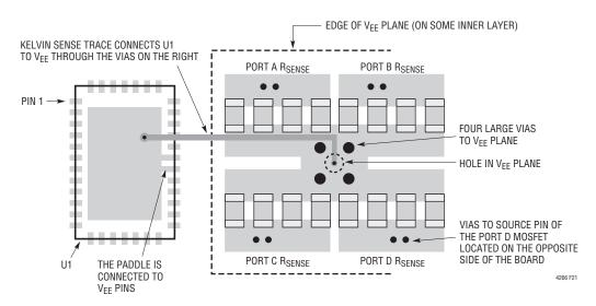
Figure 21. Good PCB Layout Example
