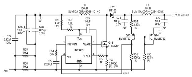
Figure 17. Positive V<sub>DD</sub> Boost Converter
