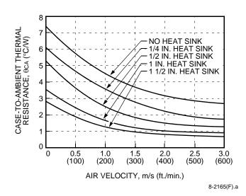
Figure 24. Case-to-Ambient Thermal Resistance Curves; Transverse Orientation
