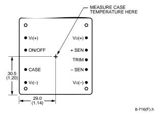
Note: Top view, pin locations are for reference only. Measurements are shown in millimeters and (inches).
