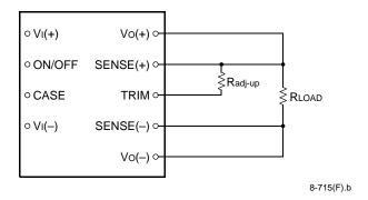
Figure 17. Circuit Configuration to Increase Output Voltage
