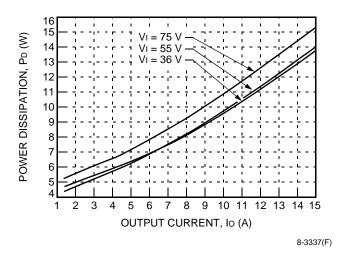
Figure 20. JAW075A Power Dissipation vs.
