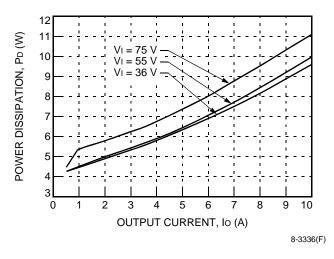
Figure 19. JAW050A Power Dissipation vs.
