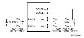
Figure 15. Effective Circuit Configuration for Single-Module Remote-Sense Operation
