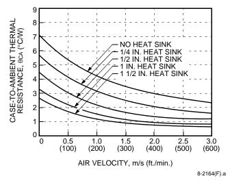
Figure 23. Case-to-Ambient Thermal Resistance Curves; Longitudinal Orientation
