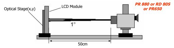
[ Figure 8 ] Optical characteristic measurement equipment and method
