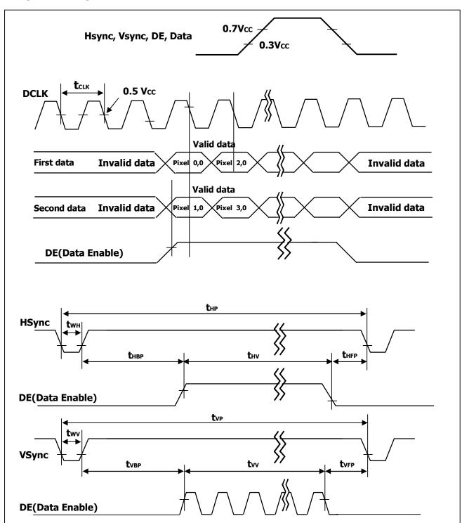
[ Figure 5 ] Signal timing waveforms
