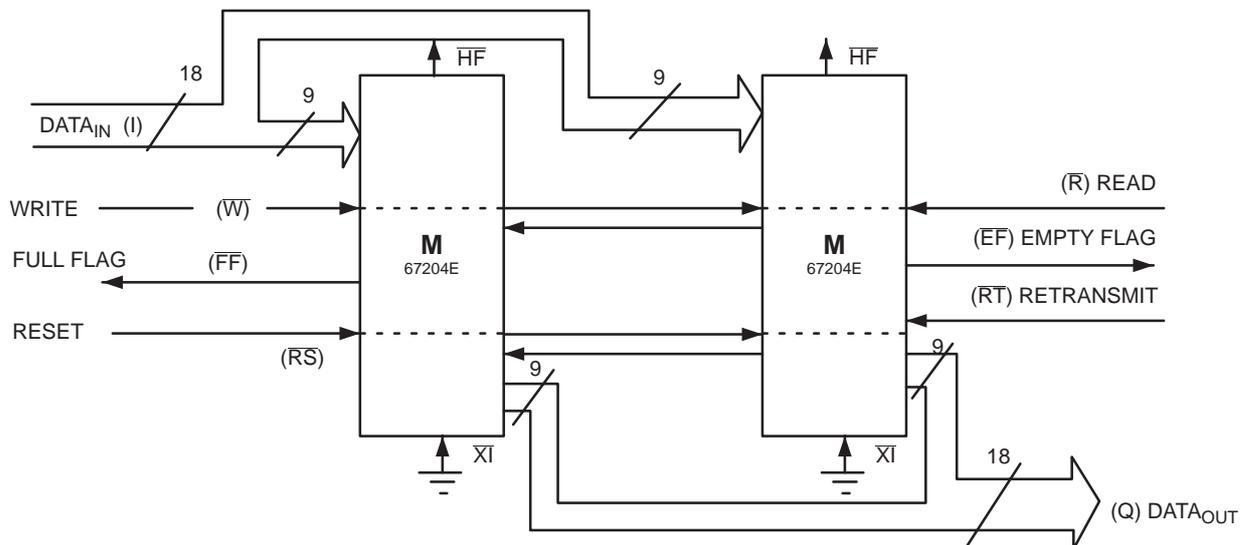
**Note :** 3. Flag detection is accomplished by monitoring the  $\overline{FF}$ ,  $\overline{EF}$  and the  $\overline{HF}$  signals on either (any) device used in the width expansion configuration. Do not connect any output control signals together.
