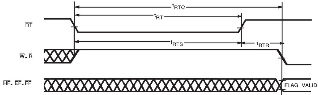
Notes : 23.  $\overline{EF}$ ,  $\overline{FF}$  and  $\overline{HF}$  may change status during Retransmit, but flags will be valid at  $t_{RTC}$ .
