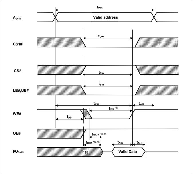
Note 16. t<sub>WP</sub> is the interval between write start and write end.
