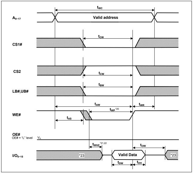
Note 20. t<sub>WP</sub> is the interval between write start and write end.
