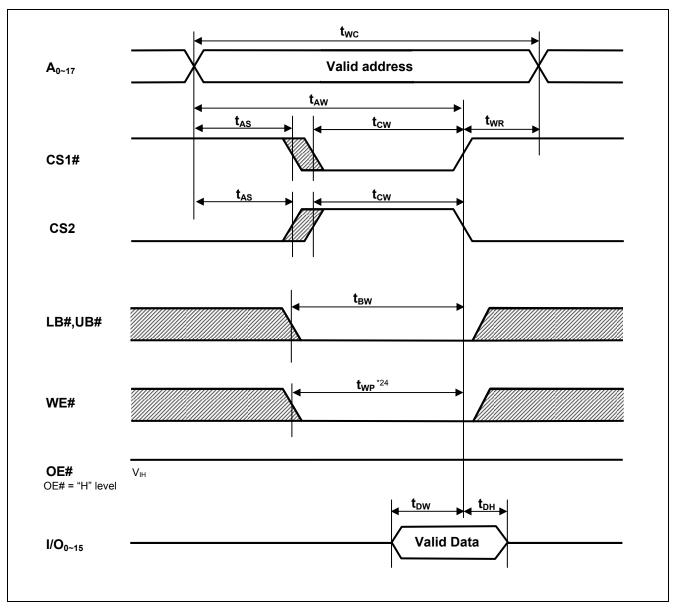
Note 24. twp is the interval between write start and write end.
