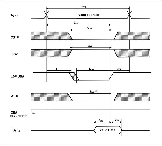
Note 25. t<sub>WP</sub> is the interval between write start and write end.
