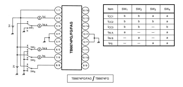
All terminals of INA, INB, and PS should output low or be connected to the ground terminal in measuring  $I_{CC3}$ .
