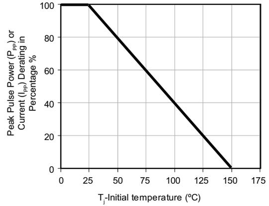
**Fig.2 PEAK PULSE POWER OR CURRENT DERATING CURVE**
