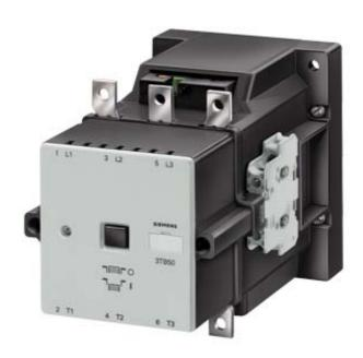
CONTACTOR SIZE 6 3-POLE AC-3 55KW, 400/380V AUXILIARY CONTACTS 21 (2NO+1NC) SETTING RANGE 0.7 TO 1.25X US SWITCHED WITH VARISTOR DC OPERATION DC SOLENOID SYSTEM DC 24V
