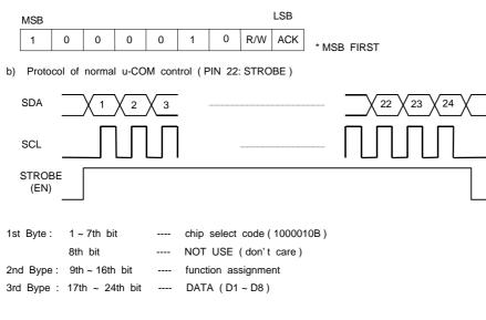
The module address of KB22688 in normal u-COM control mode is as follows.
