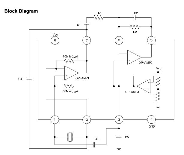
Note: Some of the functional blocks, circuits, or constants in the block diagram may be omitted or simplified for explanatory purpose.
