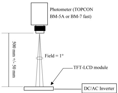
Optical characteristics measuring configuration
