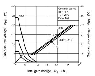
Fig. 8.1.10 Dynamic Input/Output Characteristics
