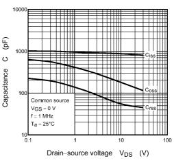
Fig. 8.2.8 Capacitance - VDS
