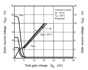
Fig. 8.2.10 Dynamic Input/Output Characteristics
