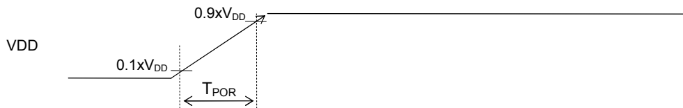
Power-on reset activation power rise time ( T_{POR} )
