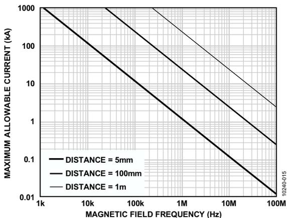
Figure 15. Maximum Allowable Current for Various Current-to-ADuM7240/ADuM7241 Spacings
