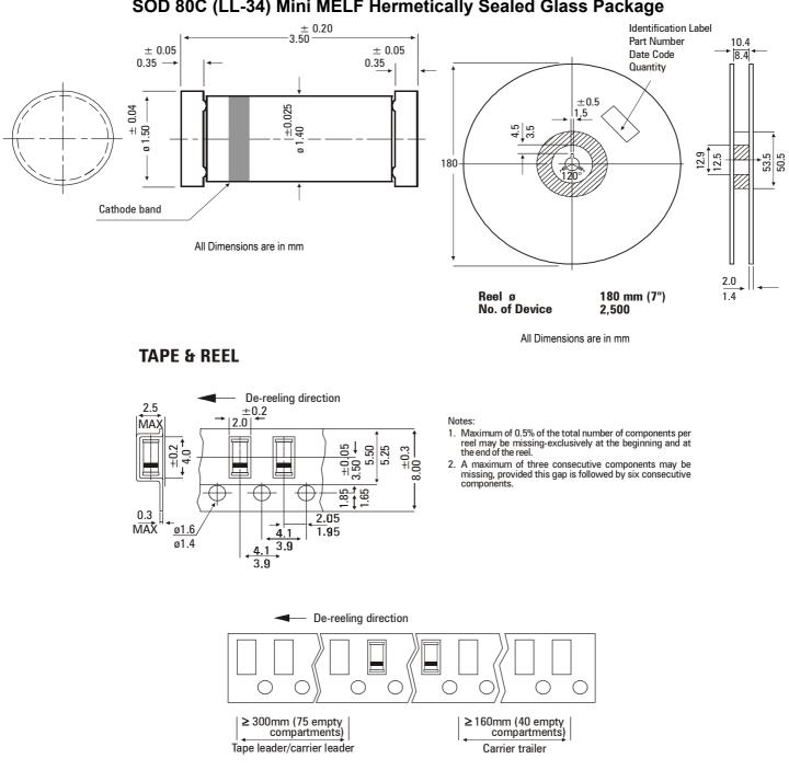
SOD 80C (LL-34) Mini MELF Hermetically Sealed Glass Package
