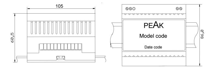
Case material is for the top cover (Lexan), lower case (Noryl) . Class UL94V0 Top cover includes ventilating louvers for cooling by air convection
