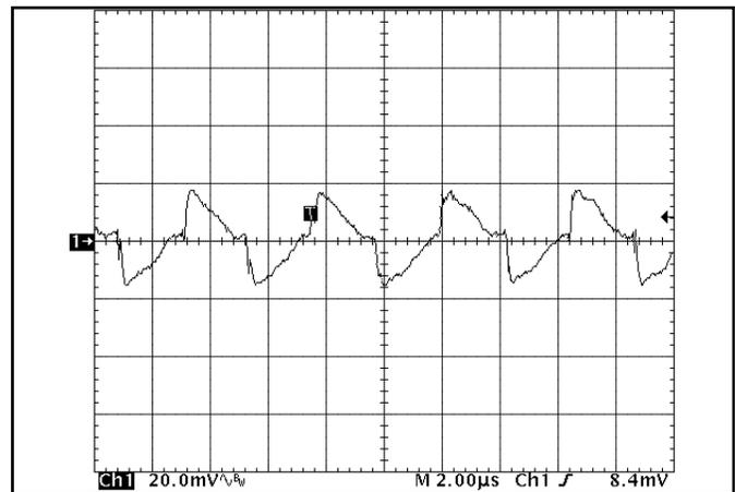
**Figure 20:** Output voltage ripple at nominal input voltage and rated load current (20 mV/div). Load capacitance:  $1\ \mu\text{F}$  ceramic capacitor and  $10\ \mu\text{F}$  tantalum capacitor. Bandwidth: 20 MHz. See Figure 17.
