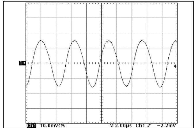
**Figure 18:** Input Terminal Ripple Current,  $i_c$ , at full rated output current and nominal input voltage with  $10\ \mu\text{H}$  source impedance and  $47\ \mu\text{F}$  electrolytic capacitor (500 mA/div). See Figure 17.
