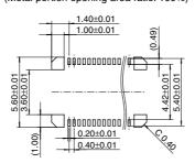
Recommended metal mask pattern Metal mask thickness: When 120 μm (Terminal portion opening area ratio: 66%) (Metal portion opening area ratio: 100%)
