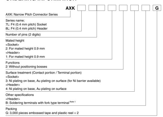
Notes: 1. "B" in the 11th digit of the header part number signifies a fork type soldering terminals to lessen the constraint on amount of solder when mounting, and a construction that makes it difficult when mounting for excess solder to interfere with the socket.
