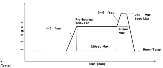
onally there is a brightness decrease caused by the influence of heat or ambient atmosphere during air reflow. It is recommended that the User use the nitrogen reflow method.
