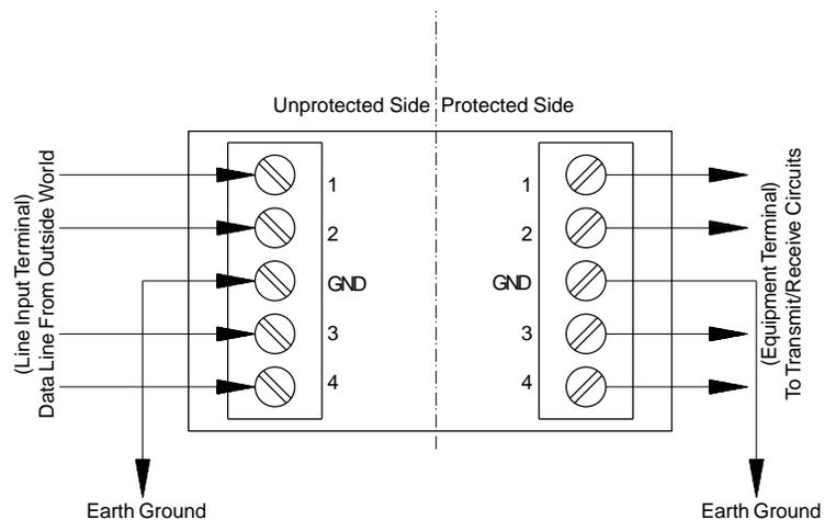
**Note:** Both ground terminals are common. Use second ground wire to reduce impedance on long runs to earth ground connections
