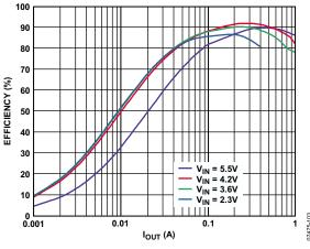
Figure 5. Efficiency vs. Output Current, PWM Mode ( $V_{OUT} = 5.0 V$ )
