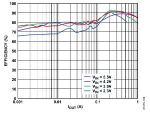
Figure 10. Efficiency vs. Output Current, PSM and PWM Mode ( $V_{OUT} = 2.8 V$ )
