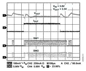
Figure 19. Load Transient (V<sub>IN</sub> = 3.6 V, V<sub>OUT</sub> = 3.3 V, I<sub>OUT</sub> = 10 mA to 300 mA)
