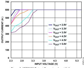
Figure 3. ADP2503 Output Current vs. Input Voltage
