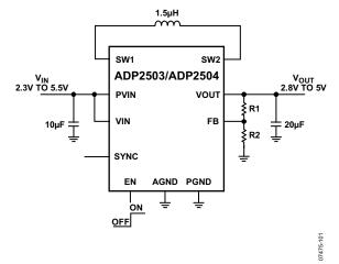
Figure 30. Typical Application Circuit for the Adjustable ADP2503/ADP2504
