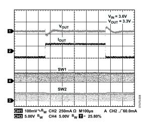
Figure 18. Load Transient ( $V_{IN} = 3.6 V$ ,  $V_{OUT} = 3.3 V$ ,  $I_{OUT} = 100 \text{ mA to } 350 \text{ mA}$ )
