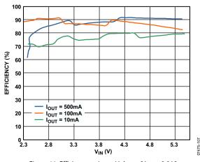
Figure 11. Efficiency vs. Input Voltage (Vout = 3.3 V)
