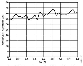
Figure 14. Quiescent Current vs. Input Voltage (Vout = 3.3 V)
