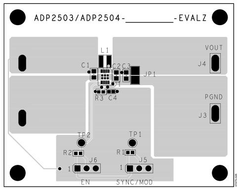
Figure 31. ADP2503/ADP2504 Evaluation Board for Fixed Output Voltages
