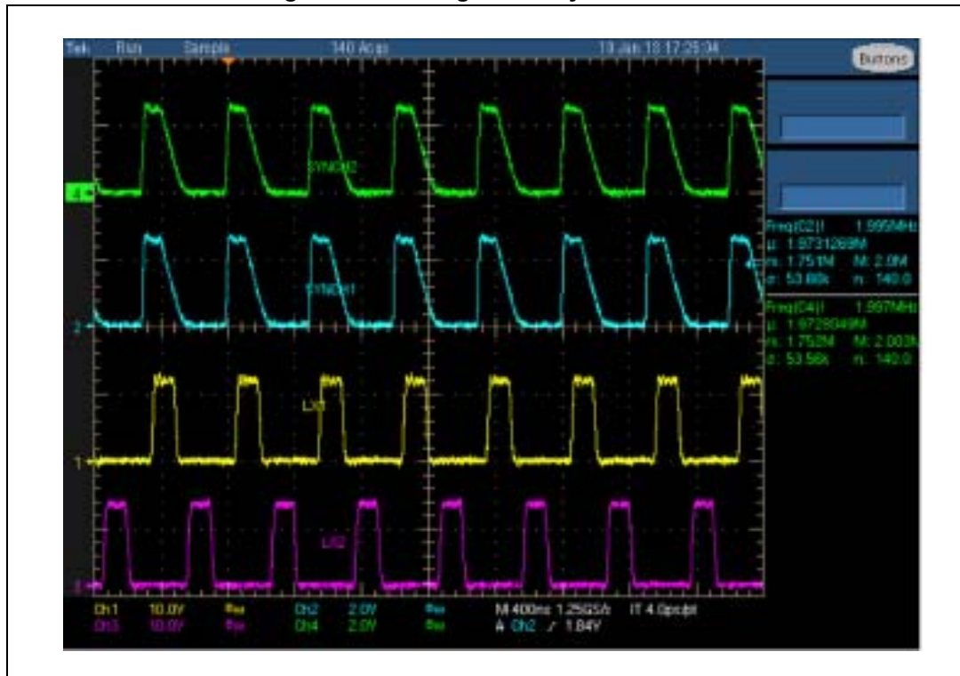
Figure 29. Two regulators synchronized
