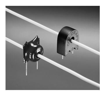
These sensors function as the secondaries of a current transformer. The conductor carrying the current to be measured is the "one turn primary." Voltage per Ampere can be adjusted by varying the terminating resistor (see note 3). Applications include sensing branch circuit overload, switcher feedback, and detecting load drop or shutdown.
