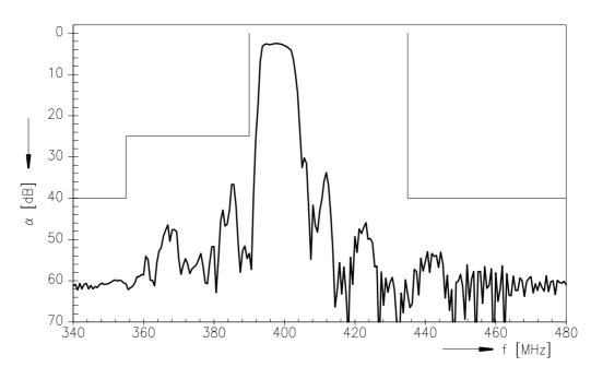
Normalized transfer function (pass band; +15 °C ... +35 °C)
