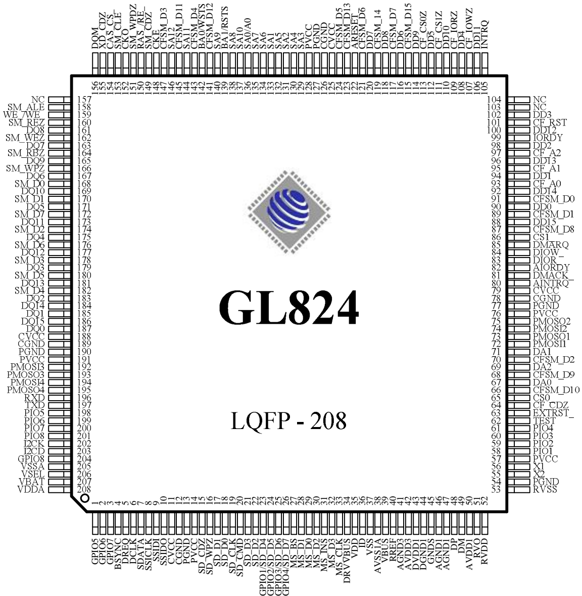
Figure 3.1 - 208 Pin LQFP Pinout Diagram
