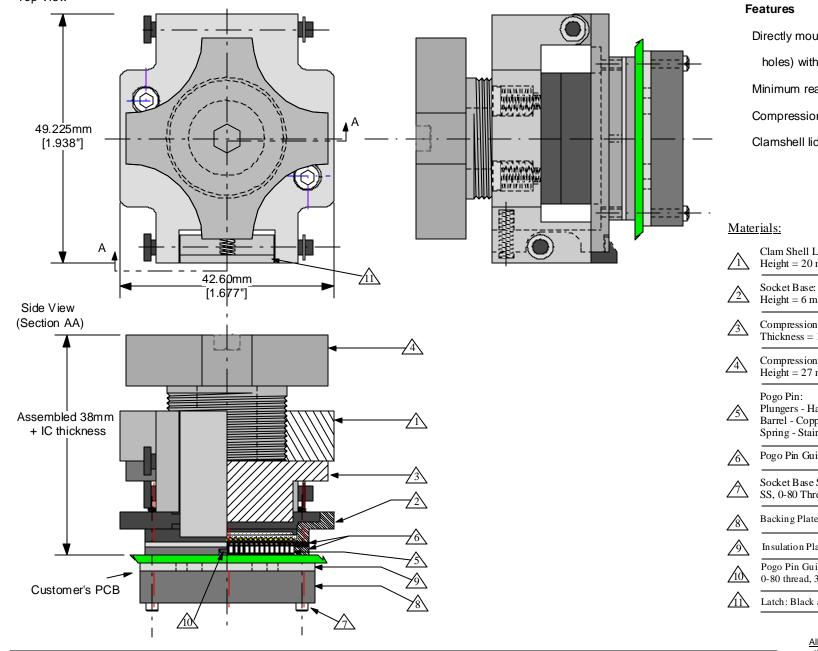
Directly mounts to target PCB (needs tooling
