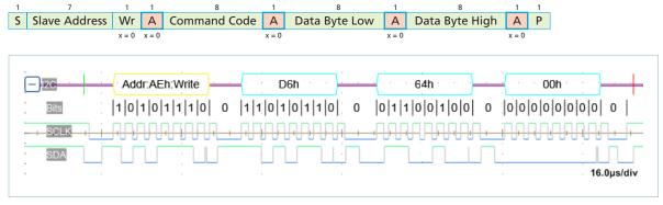
Figure 3 — TON\_DELAY COMMAND (60h)\_WRITE WORD PROTOCOL
