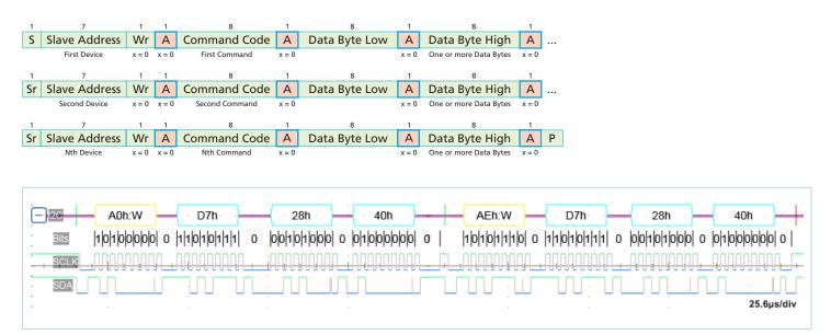
Figure 7 — DISABLE\_FAULT COMMAND (D7h)\_WRITE
