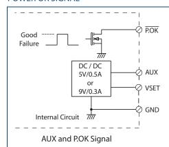
\* Place an additional capacitor to have a better performance of auxiliary power operation.
