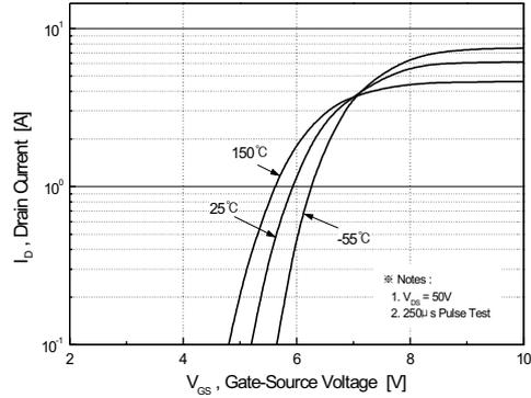
Figure 2. Transfer Characteristics
