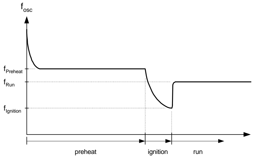
Figure 6: Oscillator frequency versus time, Normal operating conditions
