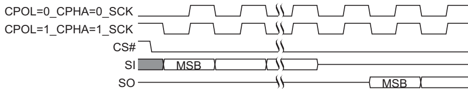
Figure 4. SPI SDR Modes Supported
