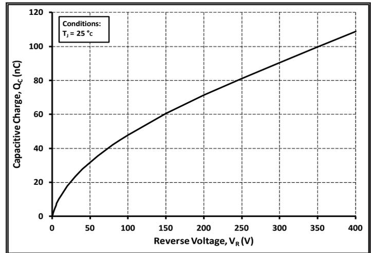
Figure 4. Typical Recovery Charge vs. Reverse Voltage
