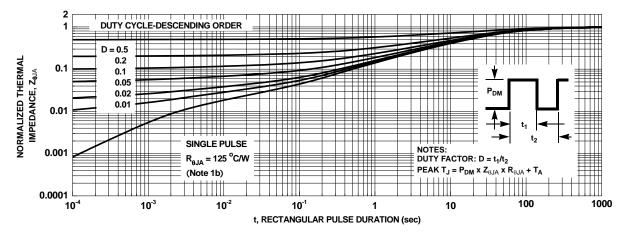
Figure 13. Junction-to-Ambient Transient Thermal Response Curve
