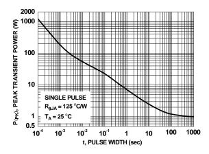
Figure 12. Single Pulse Maximum Power Dissipation
