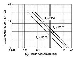
Figure 9. Unclamped Inductive Switching Capability
