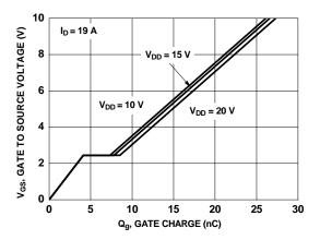
Figure 7. Gate Charge Characteristics
