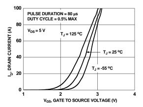
Figure 5. Transfer Characteristics
