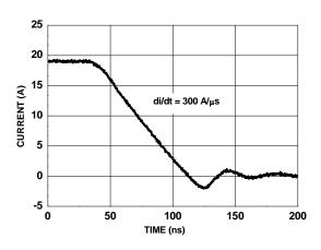
Figure 14. FDMS8026S SyncFET body diode reverse recovery characteristic
